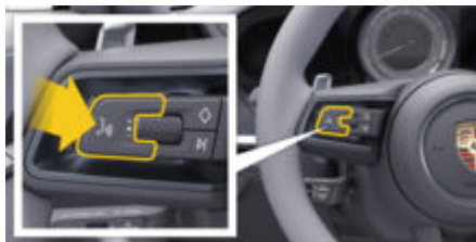
Fig. 15: Steering wheel with voice control button
