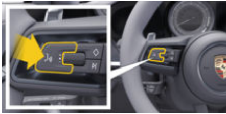
Fig. 4: Voice control button on the steering wheel
