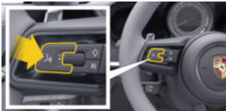
Fig. 2: Voice control button on the steering wheel
