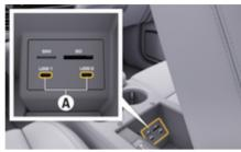
Fig. 2: USB interface (type C) in armrest
