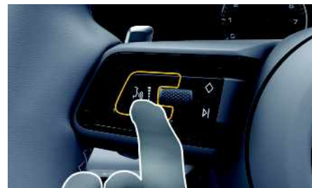
Fig. 5: Voice control button on the steering wheel
