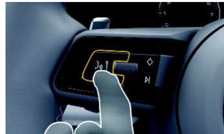
Fig. 11: Voice control button on the steering wheel
