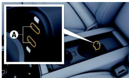
Fig. 3: USB interface (type C) in the rear center armrest
