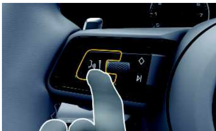
Fig. 14: Voice control button on the steering wheel
