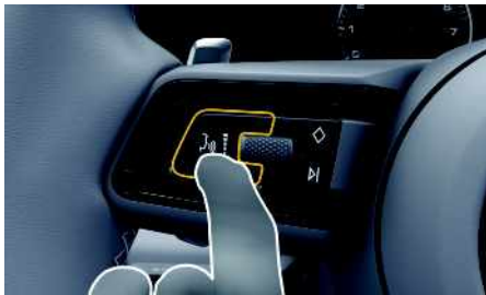
Fig. 4: Voice control button on multifunction steering wheel
